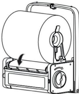
INSÉRER L'EXTRÉMITÉ DU ROULEAU DE PAPIER DANS LA FENTE D'ALIMENTATION DU DISTRIBUTEUR.
